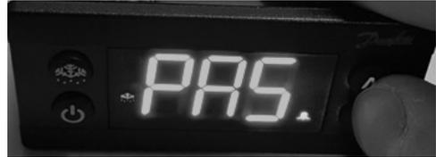
3. Scroll to **187** using the up/down arrows and push the stand-by button (lower left button) to enter.
