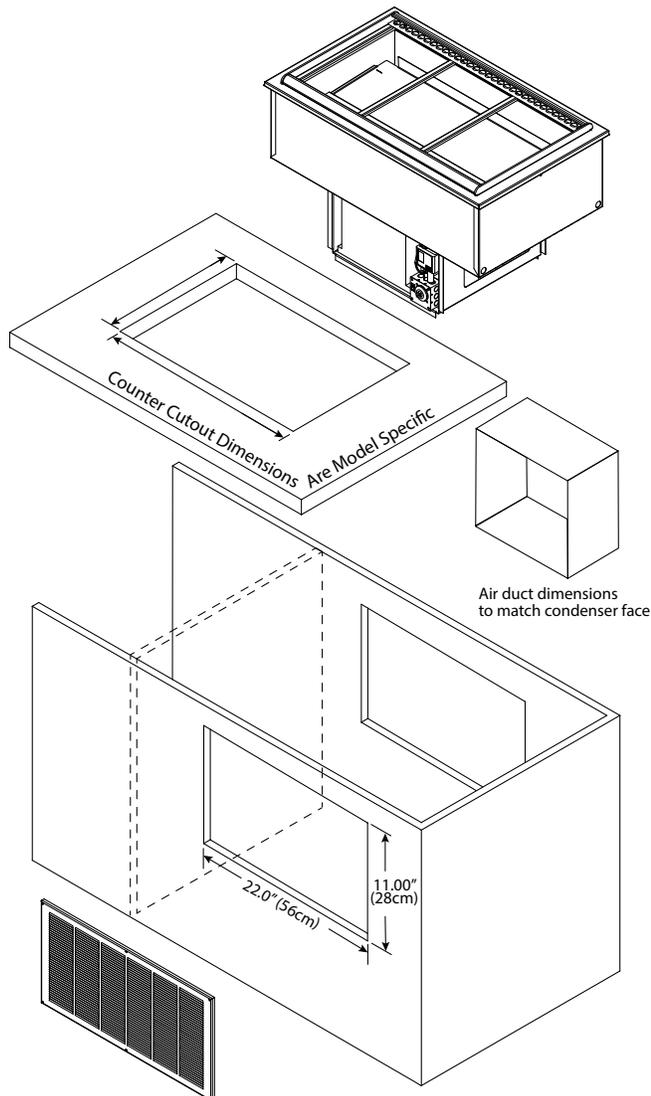
1. Install partitions between self-contained refrigerated drop-in units and other electrical appliances if they are located in the same cabinet. Partitions must fully extend front to back and top to bottom.
