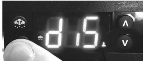
5. Scroll to **CFu** using the up/down arrows and push the stand-by button (lower left button) to enter the display unit menu.
