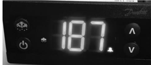
4. Scroll to **dis** using the up/down arrows and push the stand-by button (lower left button) to enter into the display menu.
