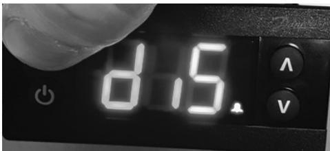
8. Push the defrost button (upper left button) to move out of the display menu and back to the normal display.
