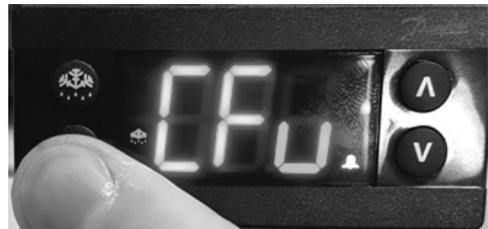
6. **-F** should be displayed indicating Fahrenheit. Use the down arrow to change it to **-C** for Celsius and hit the stand-by button (lower left button) to enter the change.
