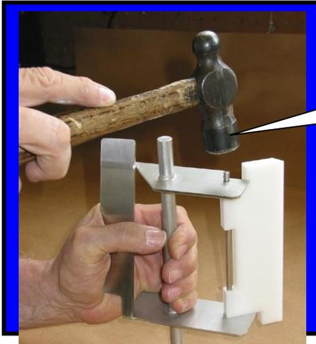
Step 2: Insert rod end into beater bar frame.
