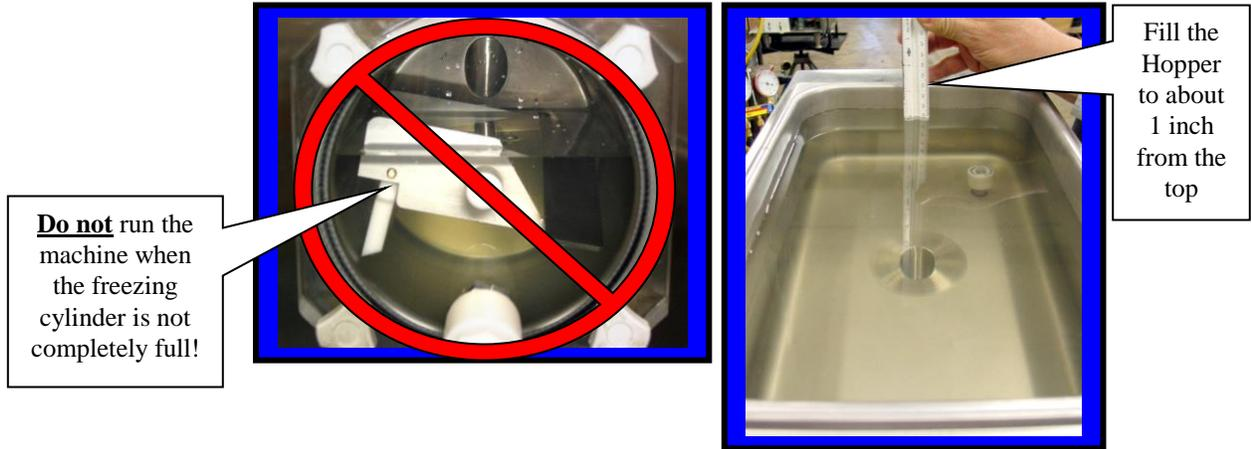
When the cylinder is full and the hopper is filled to one inch from the top, the machine is ready to run. Turn on by selecting the “right” (snowflake) position of **both** switches on the front panel.
