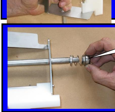
Step 5: Install spring seal F0355
