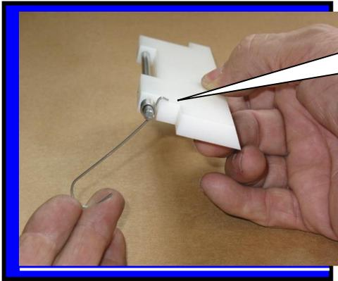
Step 1: Attach scraper blade spring F6517 as shown.
