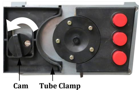
**Step 3:** Open the front door of the dispenser. Open the tube clamp by turning the cam counterclockwise.
