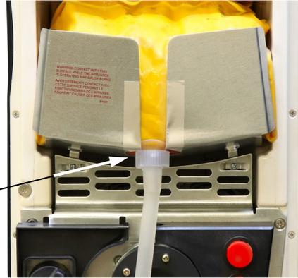
**Step 5:** Guide the tube through the pump slot from top to bottom.
