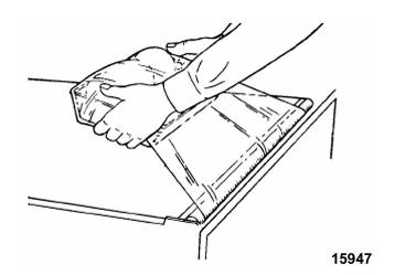
B. Pick up the package by its sides, pull it back over the cut-off rod, and then down across the cut-off rod to cut the film.
