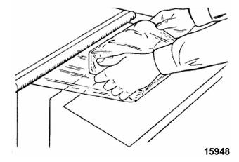
C. Stretch film over the sides and fold the excess under the package.
