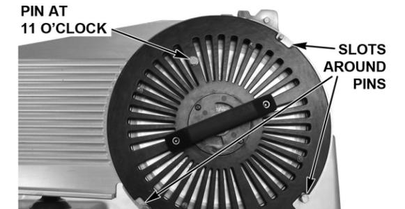
**NOTE:** If the Tool does not push the pins on the back of the Knife into the Hub, slightly nudge the Handle upwards to lock the pins into the Knife Nut.
