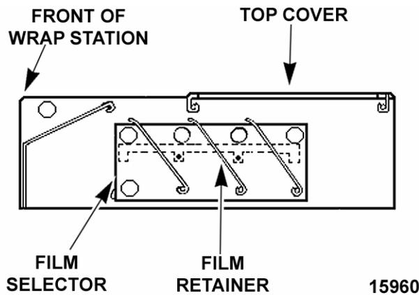
11. Raise film retainer on film selector and pull film through the film selector. Lower the film retainer to hold the film in place
