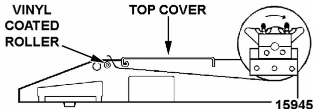
9. Raise top cover of hand wrap station to allow access to the film.
