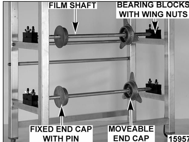
2. Rotate the upper bearing blocks to permit removal of the film shaft.
