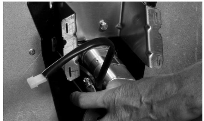
5. Grasp the gearmotor as the second pin is removed. Pivot the gearmotor out of place.
