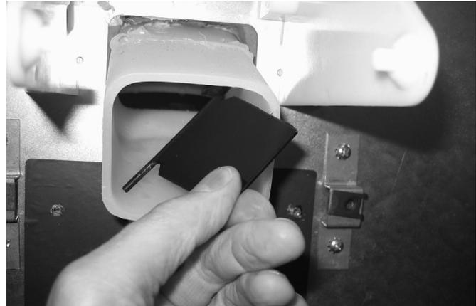
When re-assembling the rocking chute/door, the paddle wheel guard is installed inside the ice dispense snout.
