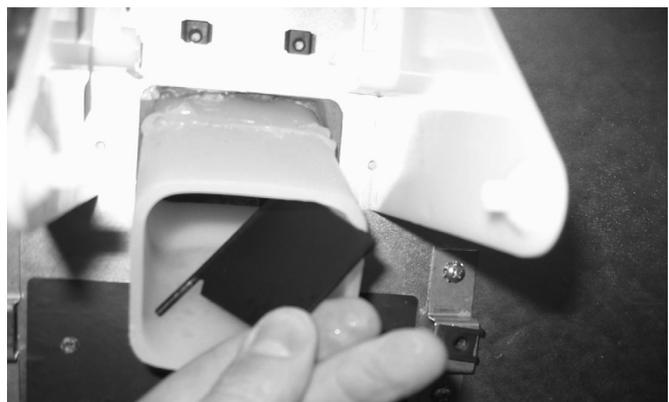
7. Pull the paddle wheel guard from the holes inside the ice dispense snout.
