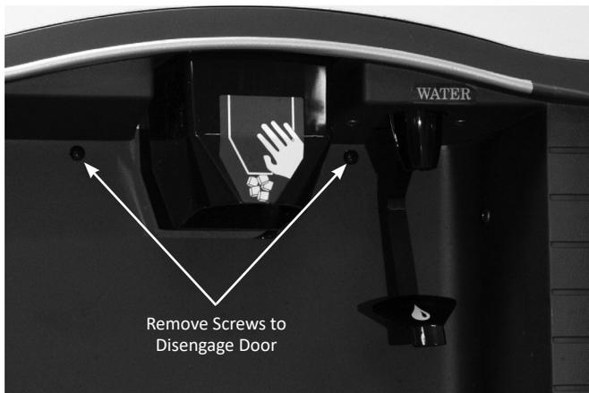
2. The 2 screws are retained by o-rings. Loosen the 2 screws with a Phillips screwdriver.
