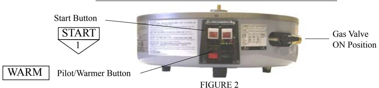
**SHUT DOWN:** When removing the pot, make sure to push the red button WARM until it clicks and is hidden by the start button. It is then in the “OFF” position. A five minute complete shutoff period is required before lighting or relighting pilot.
