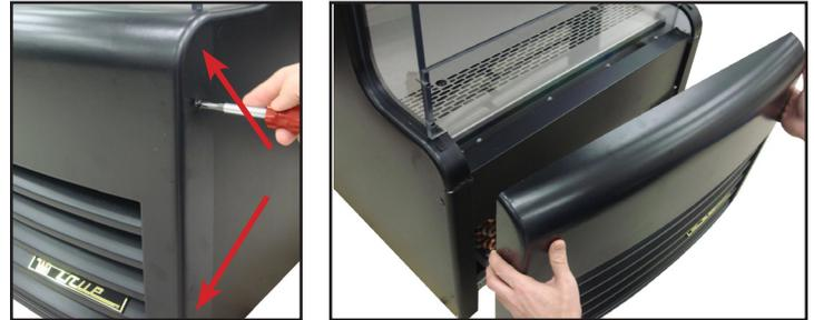
Fig. 2. TAC-14GS-LD Grill removal. Lift grill away from cabinet after removing screws.
