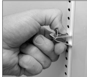
Fig. 8. You may need to squeeze or twist the bottom of the shelf clip to install.
