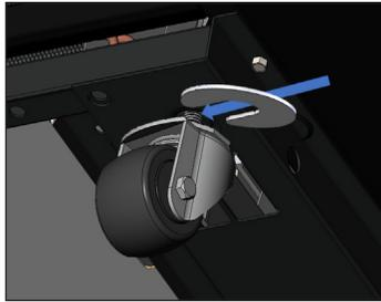
Fig. 7. Install shim(s).
