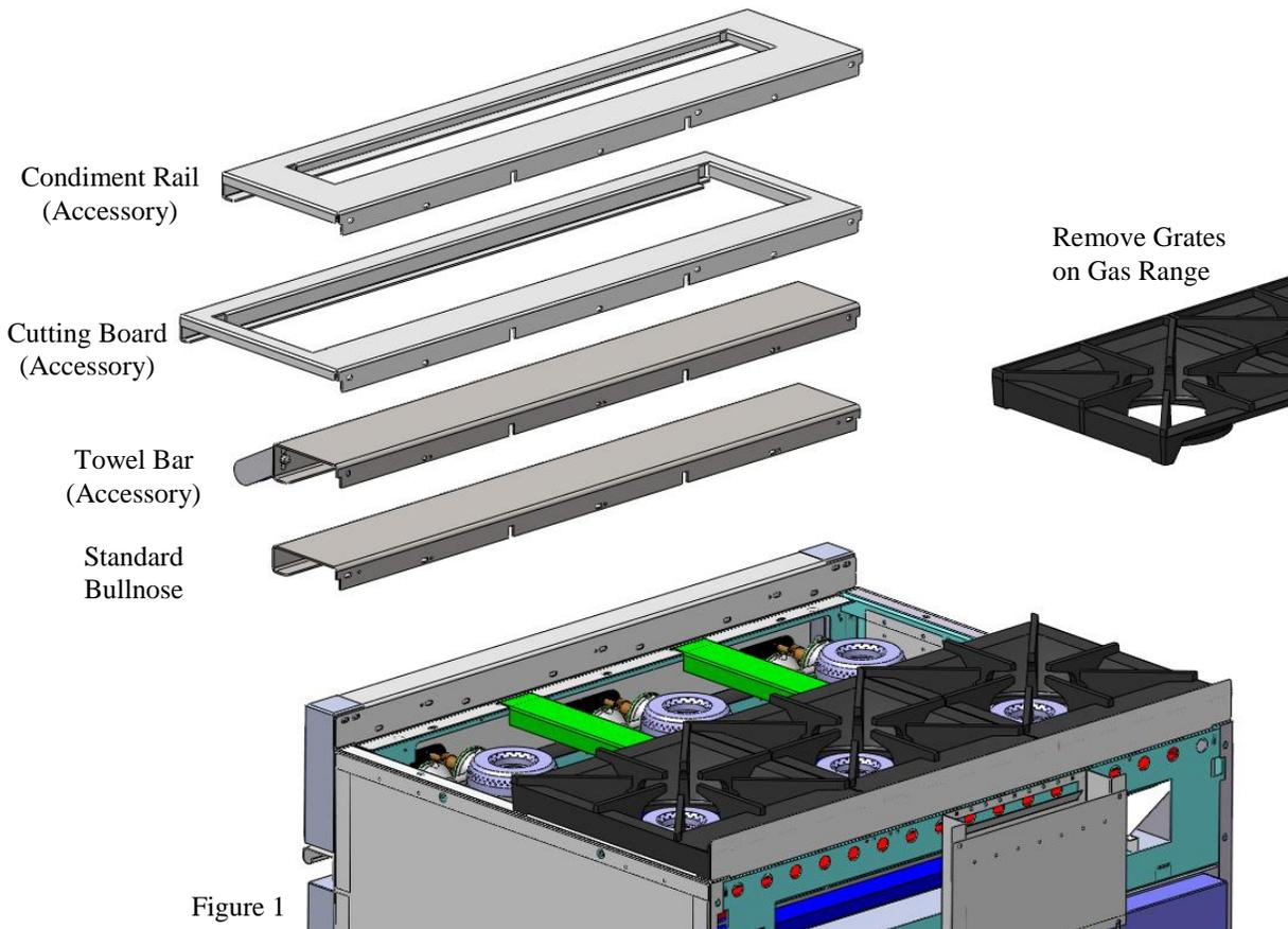
**Note:** Align the end of the Bullnose with the Range for fit.
