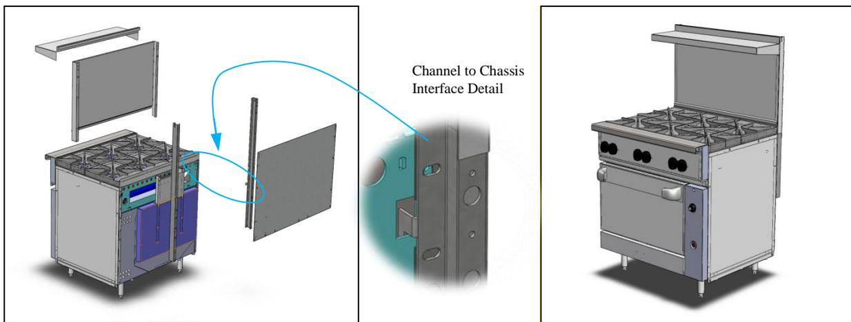
1. Engage Tab on Channels into the slots in the back of the Chassis Top (shown).
