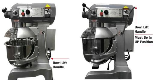
STEP 3. – The bowl lift handle must be in UP position (BDPM-30 - Rotate wheel to lift the bowl)
