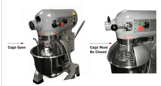
**STEP 2.** – Make sure that the bowl cage is closed completely
