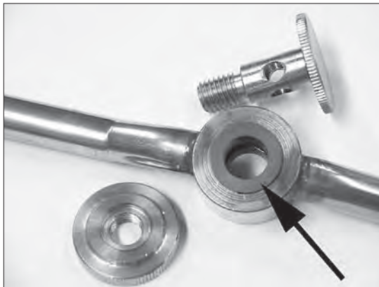
Model UH230B Only Clean the upper and lower rinse arm bearings.
