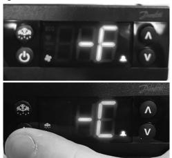
7. Push the defrost button (upper left button) to move out of the display unit menu.
