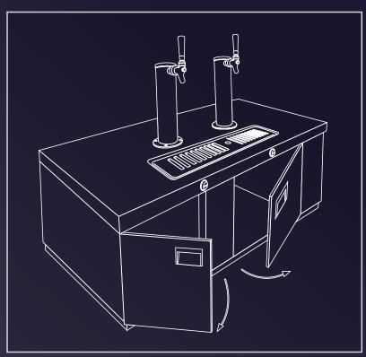
The second process is through focused draft tower cooling where a wide-diameter air hose routes refrigerated air from the evaporator housing directly into the tower receptacle. The towers are made of 304 stainless steel, heavily insulated and tightly sealed for concentrated, long term cooling.
