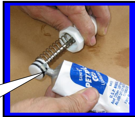
Installing O-rings onto plunger F 0491
