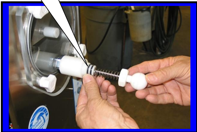
Installing Plunger assembly C6513P into faucet body
