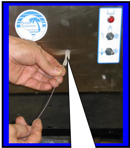
Insert long brush F6526 into drip tube
