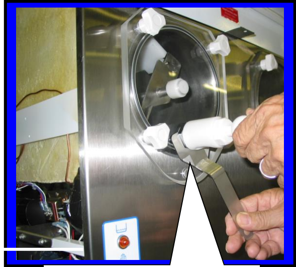
Align Faucet Assembly opening to bottom of faceplate then tighten nut
