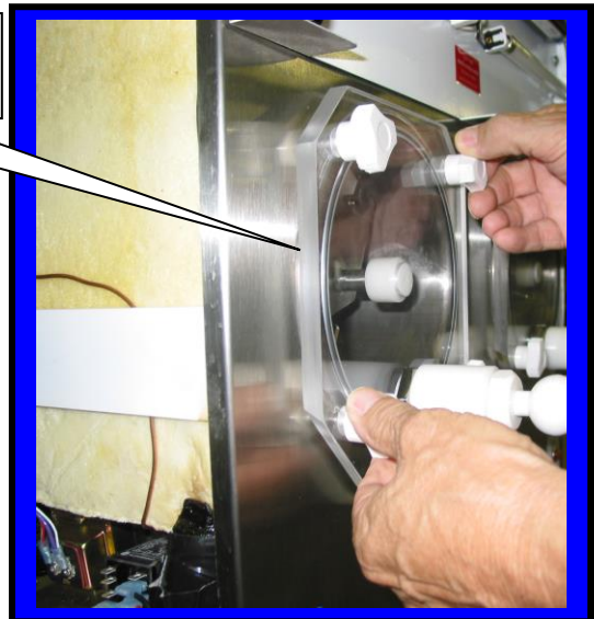
Installing faceplate C6521 onto front of Machine.
