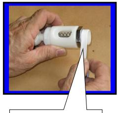
Faucet Assembly **C6513**. Teflon Tape added before installation
