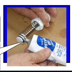
Installing Plunger assembly C6513P into faucet body
