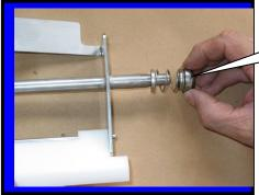
Step 5: Install spring seal **F0355**
