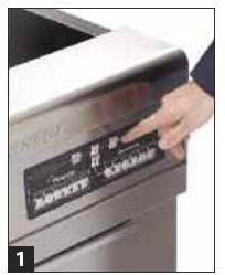
For all built-in fryers except fryers with the 3000 Controller, press OFF button to stop cooking cycle. Filtration works best when done near cooking setpoint temperature.
