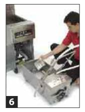
Replace hold down ring. Sprinkle one filter powder packet (1 cup) over filter paper.
