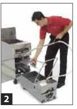
Retrieve stored portable filter and place near fryer. Remove filter pan lid. Make sure the filter pan is clean and prepared for filtering.
