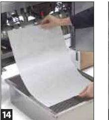
Make a good seal by placing holddown ring over filter paper securing paper evenly and completely around all sides of the filter screen.
