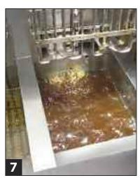
Close drain valve (red handle). Turn ON filter pump (yellow handle) and return filtered oil to the frypot. Allow oil to bubble for 15-30 seconds to clear return lines of oil.
