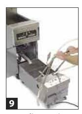
Position filter securely under the drain pipe.
