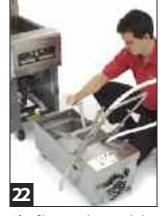
After filter parts have cooled to the touch, return the filter **screen** (making sure it is securely in place), holddown ring, crumb tray, and lid to the filter pan.
