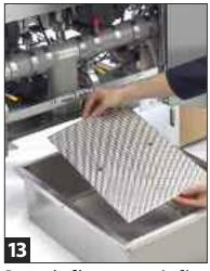
Return the filter screen to the filter pan and be sure that it is **securely**
