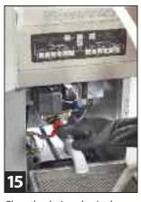
Close the drain valve (red handle). Hold the wand securely while turning on the filter pump. Return filtered oil to the frypot. Allow oil to bubble for 15-30 seconds to clear the wand hose of oil.
