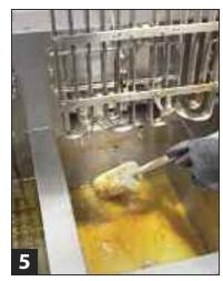
Brush crumbs from frypot with brush or scouring pad using circulating oil.
