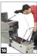
When all the oil is returned to the frypot, turn off the filter pump and unplug the filter power cord.
