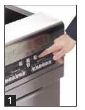
Press OFF button to stop cooking cycle. Filtration works best when done *near cooking setpoint* temperature.
