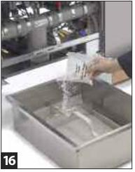
Sprinkle one filter powder packet (1 cup) over filter paper and return crumb tray.
