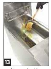
Use filter wand and frver brush to remove crumbs from frypot sides and bottom.
