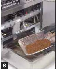
Turn off filter pump (yellow handle) and pull out filter pan. Remove, empty and wipe off crumb tray with paper towels. Discard crumbs into a fireproof container.
