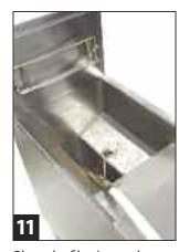
Place the filter's wand assembly securely in the frypot.
