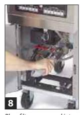
Plug filter power cord into electrical outlet. Attach drain pipe to fryer drain. Make sure drain pipe spout is pointed down.
