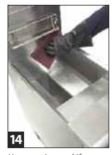
Use scouring pad if needed. Turn off filter pump. Then wipe out frypot with paper towels.
