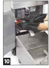
Open the drain valve (red handle) and allow oil to drain into the filter pan.
