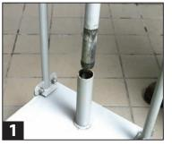
Remove the pump and pipe unit from the SDU by lifting up.
