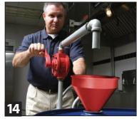
Attach hose or place funnel in oil disposal container opening. Turn pump handle toward spout to pump out oil\*.
