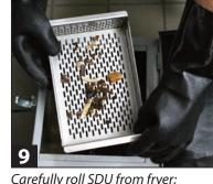
Carefully roll SDU from fryer; remove and empty crumb tray.
