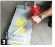
With the pump inverted turn the handle clockwise 3-4 turns stopping before oil pumps out of the spout.
