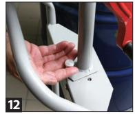
Release locking pin on pump head.
