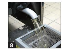
Open drain valve; drain oil into SDU; close drain valve. Remove and store drain extension.
