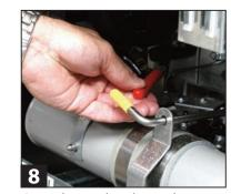
Open drain valve; drain oil into SDU; close drain valve.
