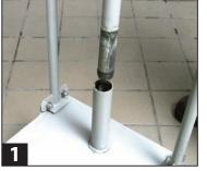
Remove the pump and pipe unit from the SDU by lifting up.
