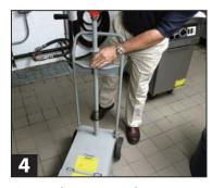
Reseat the pump and pipe unit on the SDU.
