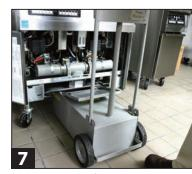
Slide SDU under filter drain down-
