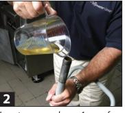
Invert pump and pour 1 cup of clean cooking oil into the pipe.
