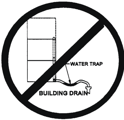
IMPROPER DRAIN LINE CONNECTION
