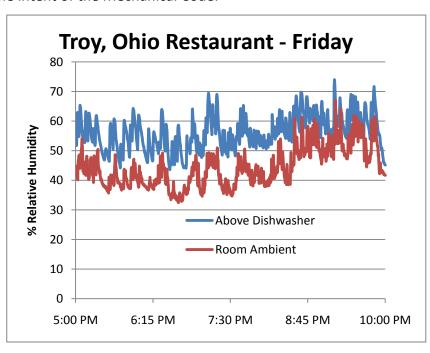
was 44.1%. While each installation is unique, the data above confirms that it is possible to operate the Ventless AM15VL in a small kitchen and still maintain the industry standard of 65% maximum relative humidity.
