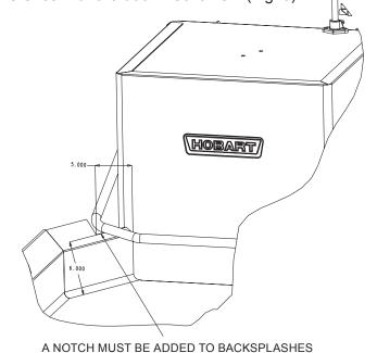
OVER 6" HIGH ON CORNER MACHINES TO PREVENT INTERFERENCE WITH DOOR MECHANISM. NOTCH MUST EXTEND 5" FROM FACE OF THE MACHINE.
