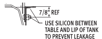
Sectional View Showing Table Connections
