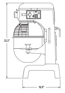
MACHINE ELECTRICAL SPECS: 120/60/1 – ETL Listed
