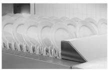
Result: more volume and versatility, quicker work. Its speed is servicer adjustable for the type of ware, soiled condition, or workforce requirements. It runs at 4 - 6.3 feet per minute.
