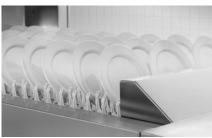
Result: more volume and versatility, quicker work. Its speed is easily adjustable on the digital display keypad for the type of ware, soiled condition, or workforce requirements. It runs at 4.0 - 8.5 feet per minute.
