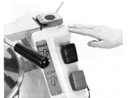
3. RELEASE START SWITCH. Machine will automatically brake to a stop. Continue pressing the start switch for as many on-off bursts as necessary.
