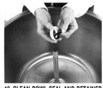
12. CLEAN BOWL SEAL AND RETAINER RING. Bowl seal and retainer ring easily snap on and off without tools. Wash if necessary, and dry. Replace and close cover.
