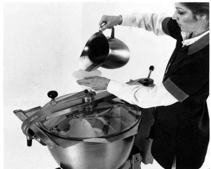
3. RELEASE START SWITCH. Machine will automatically brake to a stop. Continue pressing the start switch for as many on-off bursts as necessary.
