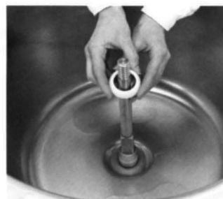
11. REMOVE BOWL SEAL AND RETAINER RING.
