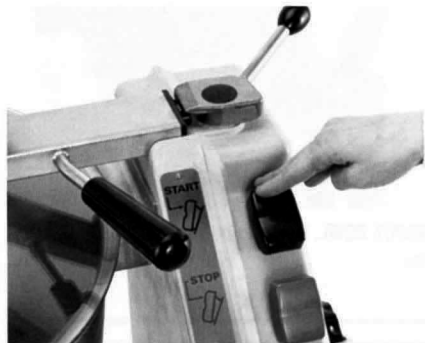
2. PRESS START SWITCH AND HOLD. Machine will run until switch is released.
