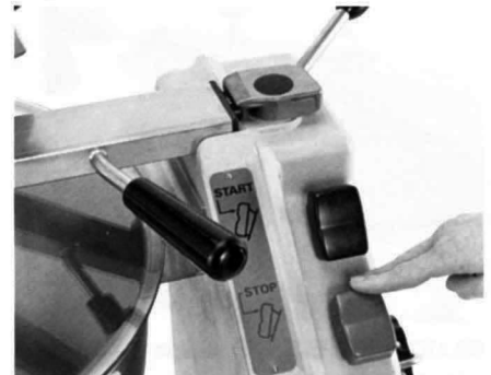
3. PRESS RED STOP BUTTON. A built-in brake will quickly stop the attachment shaft when power has been turned off.
