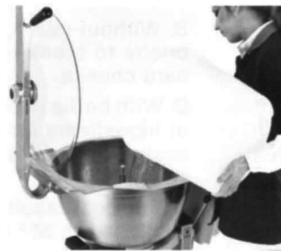
3. ADD WATER AND DETERGENT. Pour one gallon of hot water and a small amount of low-suds detergent into bowl.
