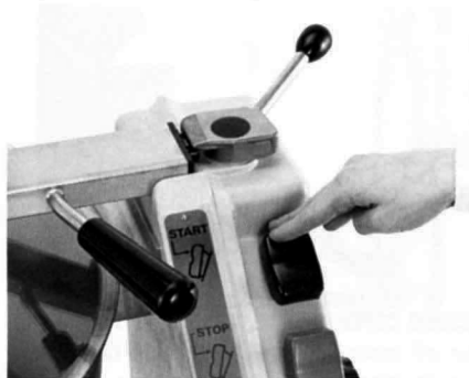
2. PRESS START SWITCH AND RELEASE. Machine will run until stop button is pressed or, until selected time has expired.
