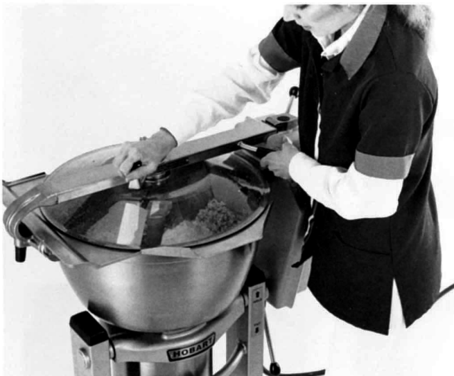
2. PRESS START SWITCH AND HOLD. Machine will run until switch is released.
