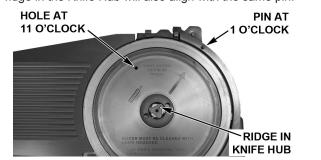
The Pin on the Knife Removal Tool fits the hole in the Knife at the 11 o'clock position.
