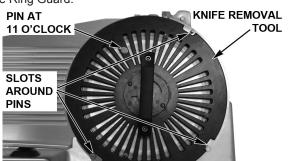
Push the Handle firmly, all the way into the hub. Then, turn the Handle counterclockwise until it stops. You may experience resistance when turning.
