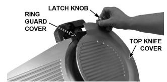
Rotate the Knife by hand to align the arrow on the Knife with the Pin on the Ring Guard at the 1 o'clock position. The ridge in the Knife Hub will also align with the same pin.
