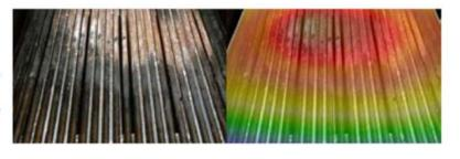
But with the burners closer together at least 6" to 4", the radiants are heating more efficiently and effectively, which will shorten the recovery time which will produce consistent cooking throughout the day. Plus it will take less BTU's per hour to maintain the proper temperature.
