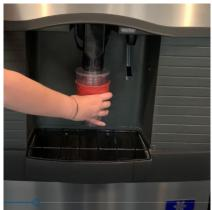
When using the Manitowoc Touchless Lever Activated Chute users are presented with improved sanitation. The lever eliminates the need to touch a hand to the machine to dispense ice. The receptacle is responsible for assisting in dispensing the ice.
