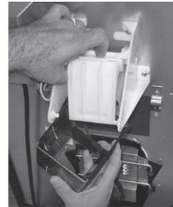
6. Put the new ice chute into place by lifting the door lock and door lock assembly. Rotate the chute counter clockwise in an up and away from you motion and snap the bracket pins into place. Replace the metal bracket clip.
