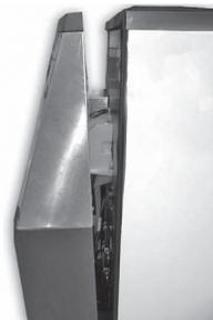
8. The Touchless ice chute is now secured. The front panel can now be pushed all the way into place.
