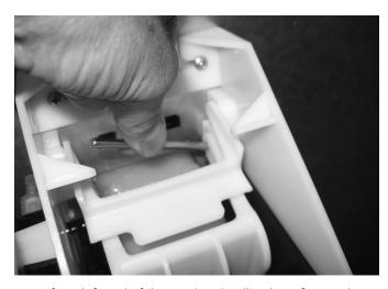
4. Lift up left end of door rod and pull rod out from right side of door.
