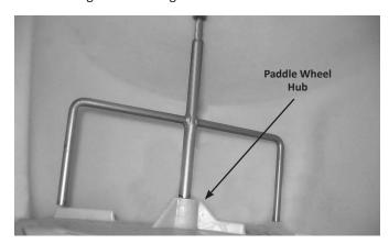
3. Push the agitator toward the back of the bin until the agitator is free of the paddle wheel hub. Remove the agitator by sliding to one side as you pull forward until the agitator shaft clears the bushing.
