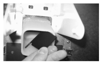
7. Pull the paddle wheel guard from the holes inside the ice dispense snout.
