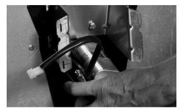
5. Grasp the gearmotor as the second pin is removed. Pivot the gearmotor out of place.
