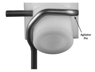
2. Pull on the hand-removable agitator pin until it is clear of the agitator bushing.
