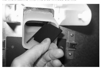
When re-assembling the rocking chute/door, the paddle wheel guard is installed inside the ice dispense snout.
