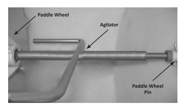
1. These parts will be removed: agitator pin, agitator and paddle wheel.
