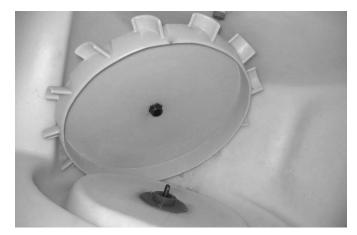
4. Slide the paddle wheel from the motor shaft and remove.
