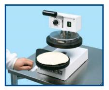
Lift up handle, open platen and place flattened crust on screen, disc or pan. Now you're ready for make-up and baking.
