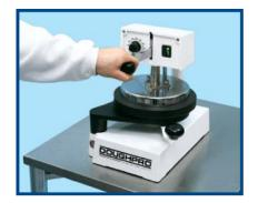
Pull down on handle and hold for about 3-7 seconds.
