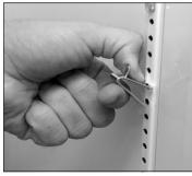
Fig. 7. The bottom tab of the shelf clip will fit tightly.
