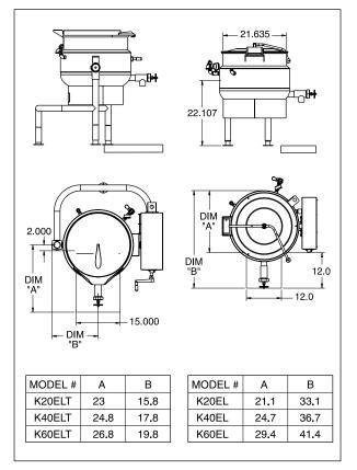
Fig 3. Floor Drain Location
